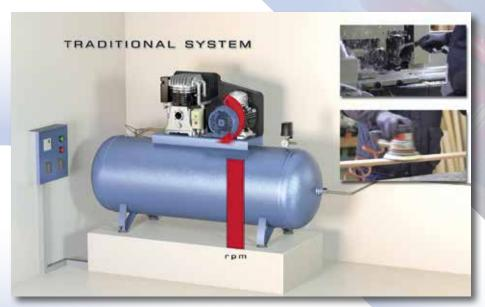
With traditional systems, the motor keeps on running and consuming at 100% of its rated speed, also during no load stage
